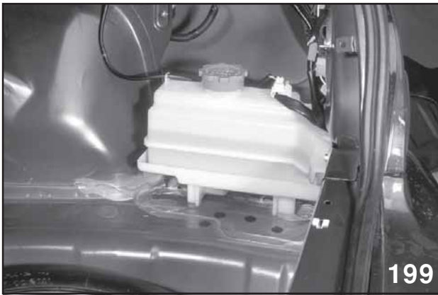
Water Tank Complete
