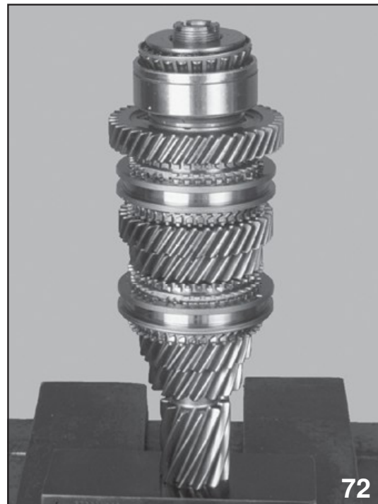
Installing Upper Bearing
