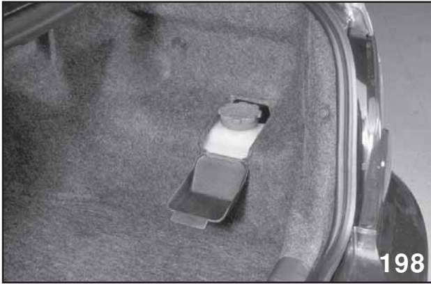
Normal Access to the Water Tank
