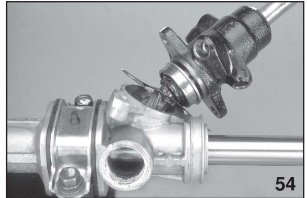
Removing Control Valve
