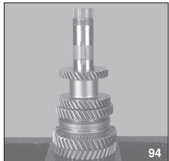
3rd/4th Gear Installed and Upper Woodruff Key
