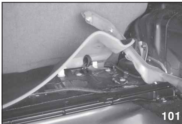
Vent Control Piping
