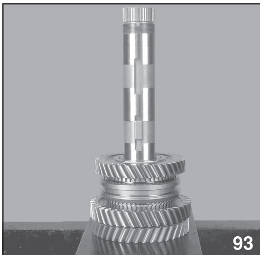
2nd Gear Installed and Lower Woodruff Key
