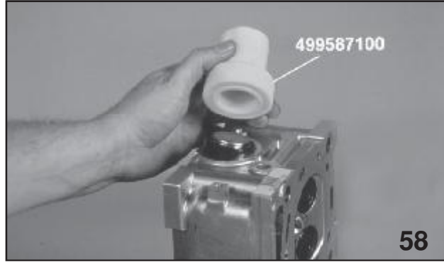
Installing the Oil Seal
