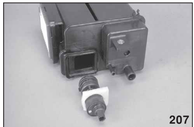
Drain Valve Separated from Canister (NOT SERVICEABLE)
