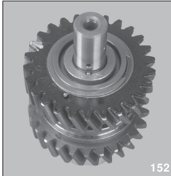
Washer and Upper Knock Pin Installed
