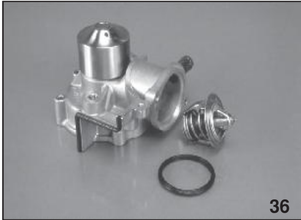
Water Pump Assembly-Cooling System
