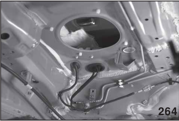
Tank Removed, Main Pump Access
