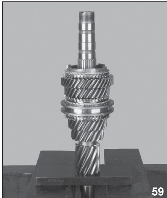
Baulk Ring Installed
