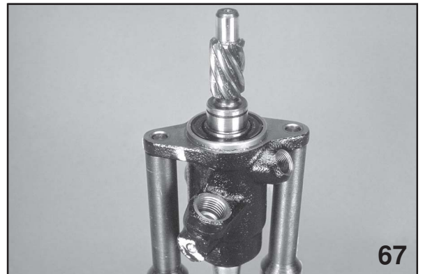
Installing Rotary Control Valve
