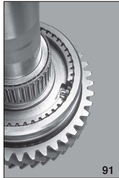
Slider and Bearing Installed
