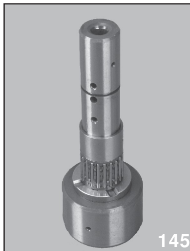
Lower Bearing and Reverse Idler Bushing Installed
