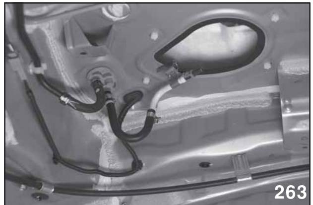
Tank Removed, Sup Pump Access
