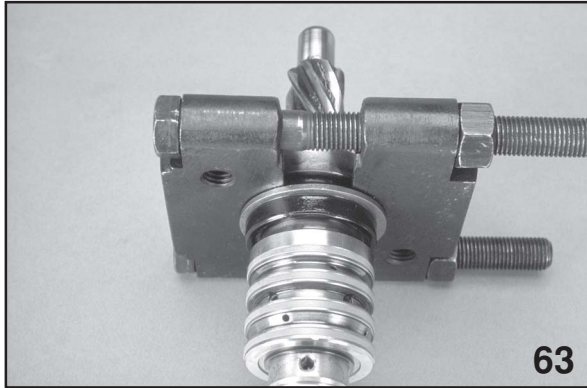
Removing Lower Bearing
