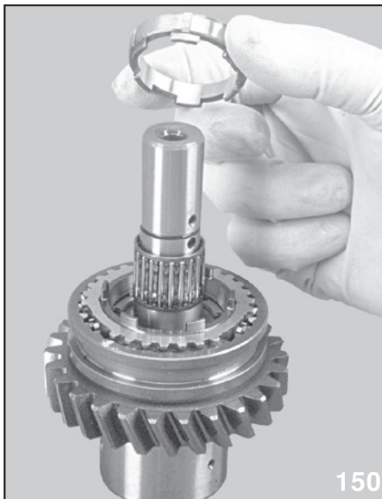
Installing Inner Baulk Ring
