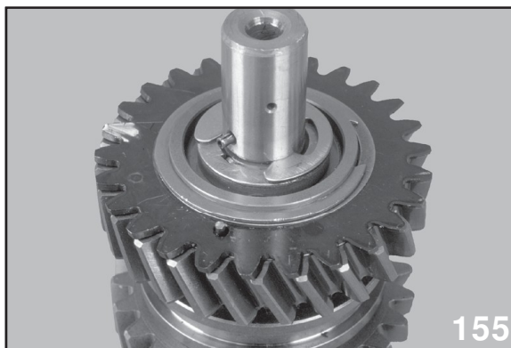
Spring Pin Installed
