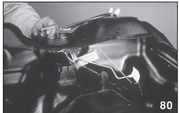
Removing Sending Unit
