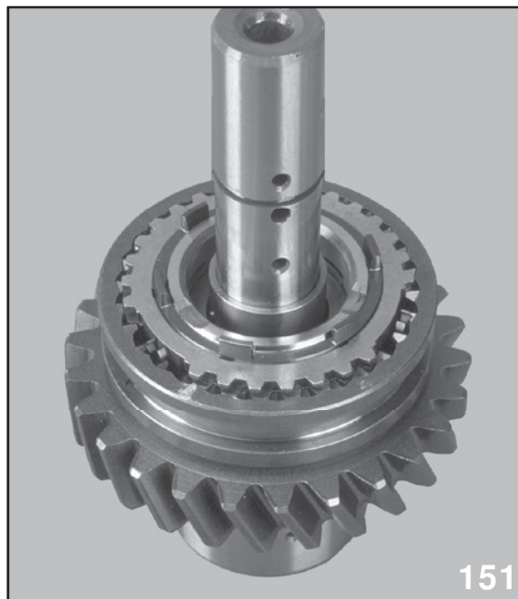
Inner Baulk Ring Installed
