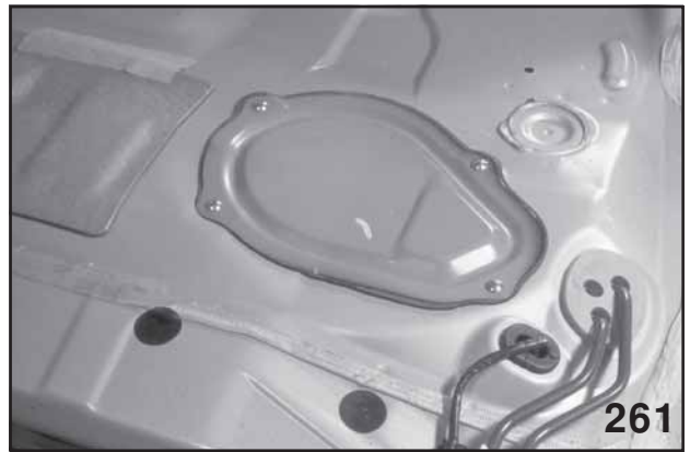
Sub Pump Access
