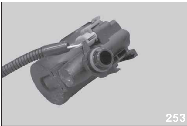
Drain Valve Separated from Canister (NOT SERVICEABLE)
