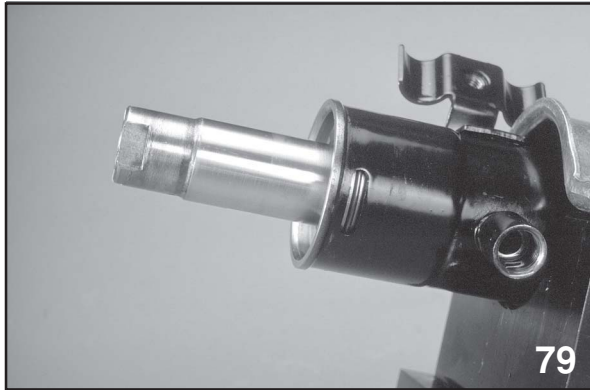
Circlip installation complete
