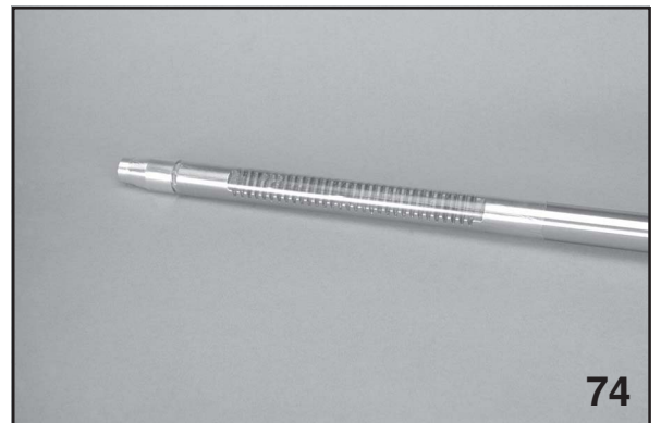
Rack Cover installed
