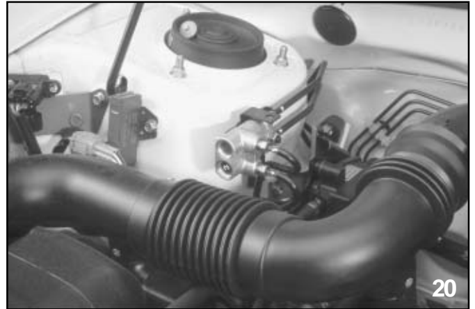
Typical proportioning valve
